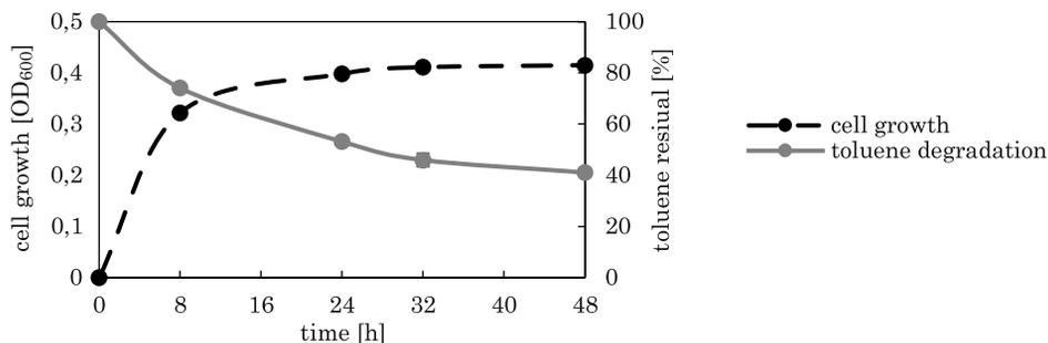
Fig. 1. Toluene-degrading and growth curves of strain ATHH39
