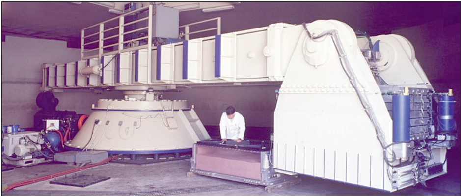
Fig. 1. Geotechnical beam centrifuge in Davis, University of California Source: KUTTER (1998).
