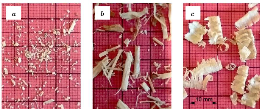
Fig. 1. Examples of the morphology of pine sawdust obtained from various cutting devices: *a* – sawdust from a band sawmill, *b* – sawdust from a frame sawmill, *c* – sawdust from a milling machine
