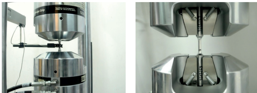
Fig. 2. Samples analyzed in MTS 810.23 load frame with a cross-sectional strain extensometer
