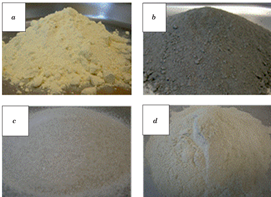
Fig. 1. Materials used in the researches: a - sulphur, b - fly ash, c - microsilica, d - zeolite
