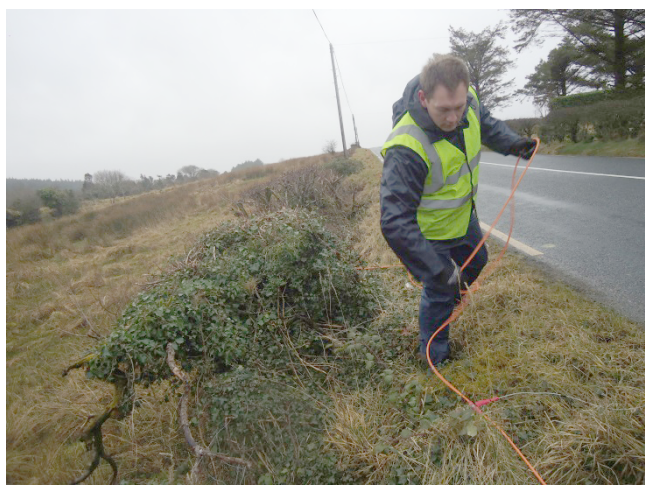
Fig. 4. Installation of one of the lines of electrical resistivity tomography profile
