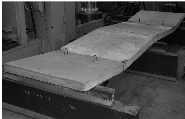
Fig. 8. Mode of failure slabs C-1 and C-2
